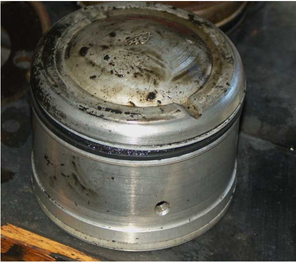
Original ATE Piston from Accumulator, source Martin Werminghausen
