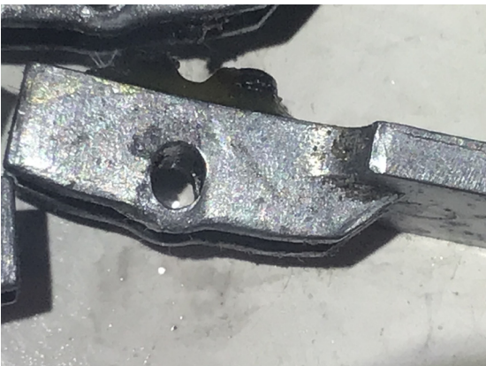
Worn out Window Switch Lever (Aluminum) , source Martin Werminghausen
