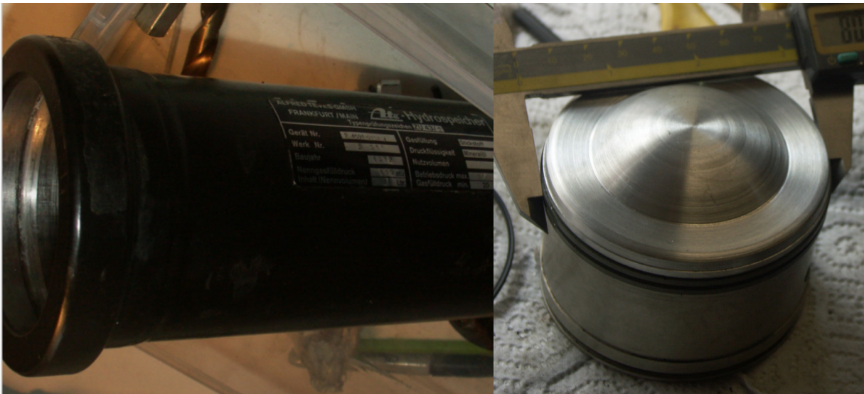
ATE Accumulator during Rebuilding, machining new Piston for modern piston seal, source Martin Werminghausen
