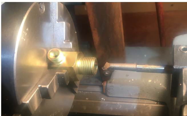
Machining during Repair of Accumulator Check Valve, source Martin Werminghausen
