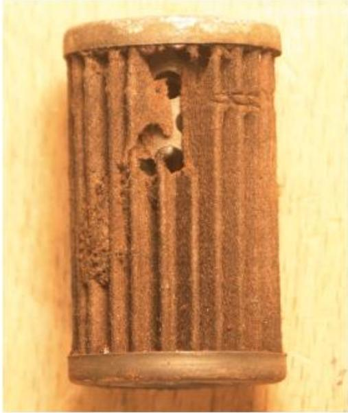
Diagram 1 Damaged Air Filter
